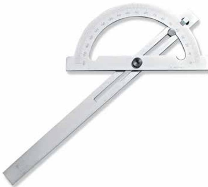
*Adjustable goniometer. Made from galvanically treated, anti-corrosion steel. Angle capacity 10 – 170° with 1° graduations. Etched, easy to read, long-lasting.*
