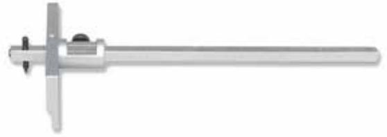
*Scribing instrument with square beam, in satin chromed-steel for machinists. Slider fit with index line. Height adjustable point with carbide tip. Base with casehardened and hardened steel sliding support. Etched graduation, easy to read and long-lasting.*
