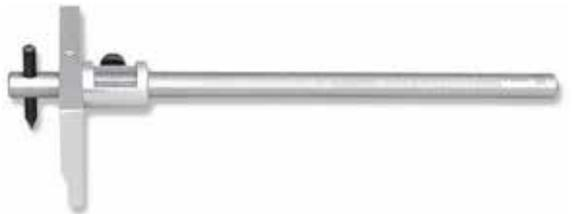
*Scribing instrument with round beam, in satin chromed-steel for machinists. Slider with index line. Height adjustable point with carbide tip. Base with casehardened and hardened steel. Etched graduation, easy to read and long-lasting.*
