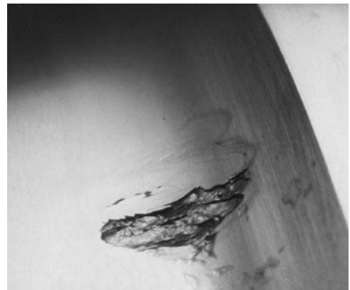
Fig. 5.2 Photo-illustration of fatigue damage on the raceway
