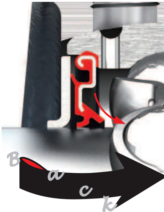
Fig. 1.3 Sealing mechanism of ball bearing units
