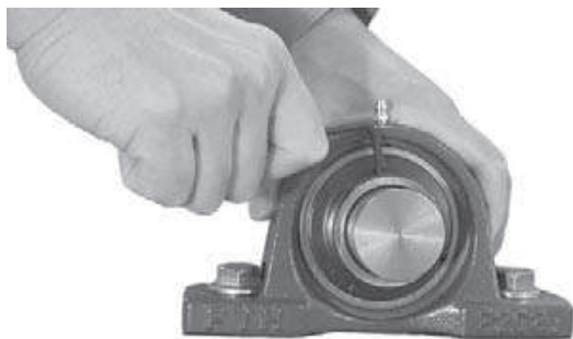
Fig. 14.5 Tightening of set screws
