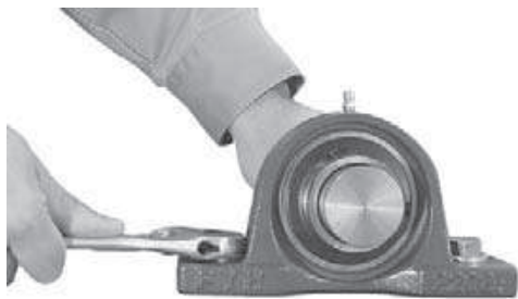
Fig. 14.4 Installation of setscrew units
