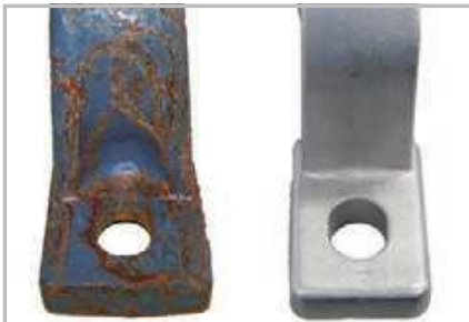
Great performance in demanding salt spray tests (72 hrs) on Stainless units
