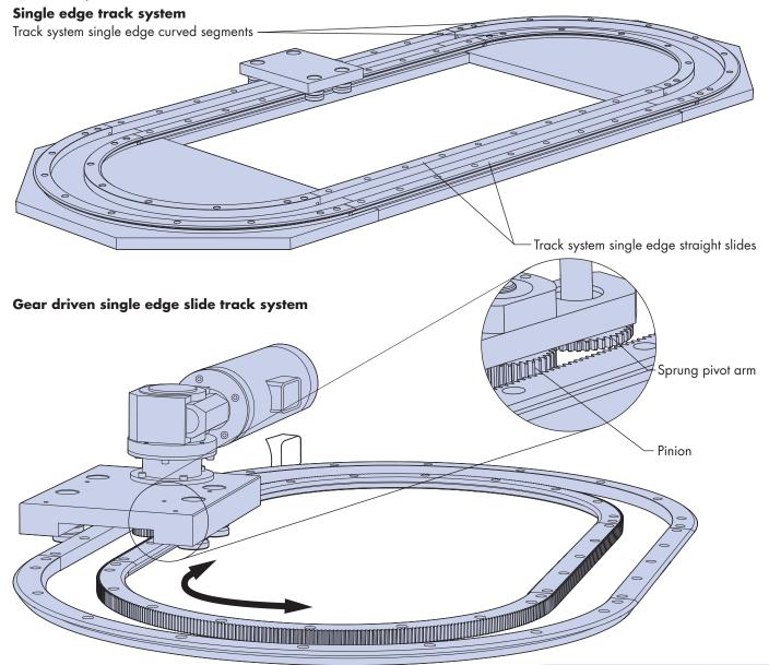
Single edge track system with a gear drive on the inner curved and straight slides, engages with a pinion driven from the motor. A sprung pivot arm ensures that the pinion remains engaged with the rack as it travels from straight to curve.
