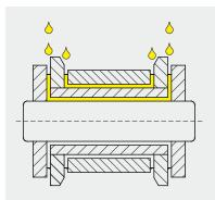
The lubricant product must be able to penetrate into the bearing area of the chain. To guarantee this the lubricant must be applied deliberately to the gap between the inner and outer plates.
