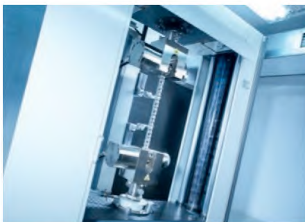
Evaluation of chain breaking strength and elongation up to 1000kN
