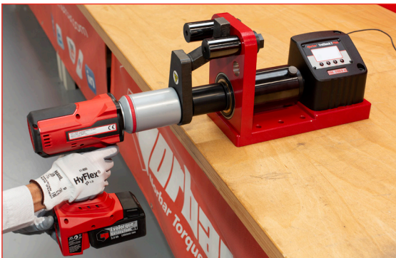
TruCheck™ 2 Plus 1100 shown with a Power Tool Test Fixture (not included - see page 27) allowing for cost-effective checking of power tools
