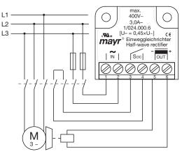
DC-side switching means short brake engagement times (e.g. for EMERGENCY STOP operation); however, louder switching noises.
