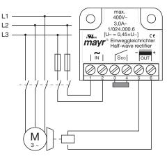
AC-side switching means low-noise switching; however, the brake engagement time is longer (approx. 6 - 10 times longer than with DC-side switch-off), use for non-critical braking times.
