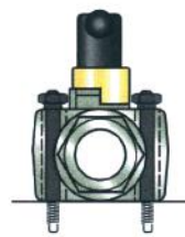
on frame fixing by studs
